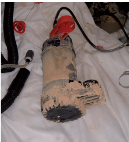
Examples of lime scale build up in cavity drain system.
